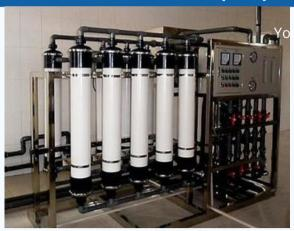
Ultrafiltration is another type of membrane filtration, which is a pressure-driven water filtration process. In the ultrafiltration process, membrane pore size plays an important role; feed water is pressed into modules through the pump, depending upon the pore size of the membranes contaminants are rejected and filtered water is taken out to the storage tank or further sent as RO feed water.
